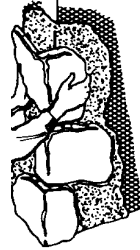
Figure 1 Apply corners— alternating long and short legs in the opposite directions.
